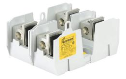
Bussmann modular fuse block, accepts J fuses, 200A, 600V, 2-pole, 6 AWG-250 MCM copper or aluminum, box lug, panel mount.
