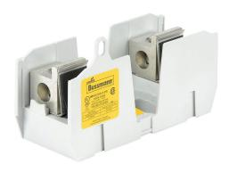
Bussmann modular fuse block, accepts J fuses, 200A, 600V, 1-pole, 6 AWG-250 MCM copper or aluminum, box lug, panel mount.
