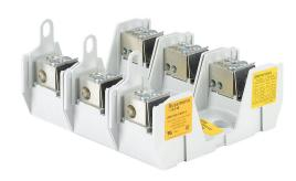
Bussmann modular power distribution fuse block, multi-wire, accepts J fuses, 100A, 600V, 3-pole, 1 line/4 load opening(s) per pole, box lug, panel mount.
