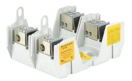
Bussmann modular power distribution fuse block, multi-wire, accepts J fuses, 100A, 600V, 2-pole, 1 line/4 load opening(s) per pole, box lug, panel mount.
