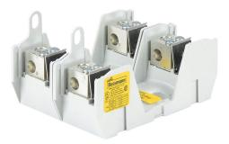
Bussmann modular fuse block, accepts J fuses, 100A, 600V, 2-pole, 14-1/0 AWG copper or aluminum, box lug, panel mount.
