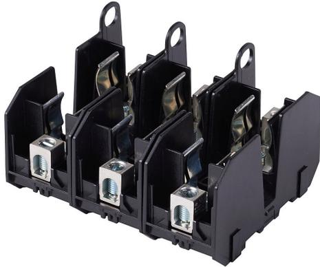
Bussmann modular fuse block, accepts J fuses, 60A, 600V, 3-pole, 14-2 AWG copper or 8-2 AWG aluminum, box lug, 35mm DIN rail or panel mount.
