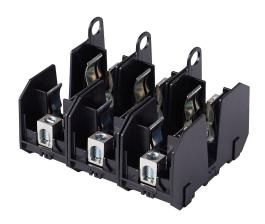
Bussmann modular fuse block, accepts J fuses, 60A, 600V, 3-pole, 14-2 AWG copper or 8-2 AWG aluminum, box lug, 35mm DIN rail or panel mount.
