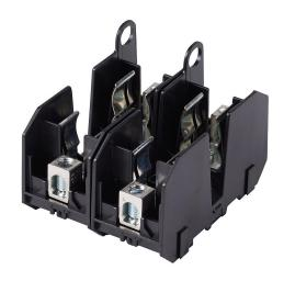
Bussmann modular fuse block, accepts J fuses, 60A, 600V, 2-pole, 14-2 AWG copper or 8-2 AWG aluminum, box lug, 35mm DIN rail or panel mount.
