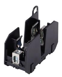
Bussmann modular fuse block, accepts J fuses, 60A, 600V, 1-pole, 14-2 AWG copper or 8-2 AWG aluminum, box lug, 35mm DIN rail or panel mount.
