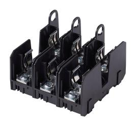
Bussmann modular fuse block, accepts J fuses, 30A, 600V, 3-pole, 18-10 AWG copper only, screw with pressure plate, 35mm DIN rail or panel mount.
