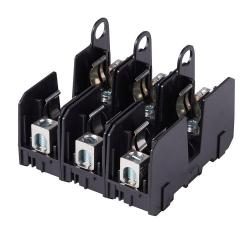
Bussmann modular fuse block, accepts J fuses, 30A, 600V, 3-pole, 14-2 AWG copper or 8-2 AWG aluminum, box lug, 35mm DIN rail or panel mount.
