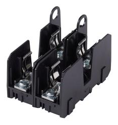
Bussmann modular fuse block, accepts J fuses, 30A, 600V, 2-pole, 18-10 AWG copper only, screw with pressure plate, 35mm DIN rail or panel mount.
