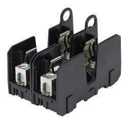
Bussmann modular fuse block, accepts J fuses, 30A, 600V, 2-pole, 14-2 AWG copper or 8-2 AWG aluminum, box lug, 35mm DIN rail or panel mount.
