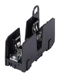
Bussmann modular fuse block, accepts J fuses, 30A, 600V, 1-pole, 18-10 AWG copper only, screw with pressure plate, 35mm DIN rail or panel mount.
