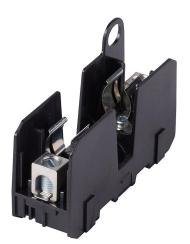
Bussmann modular fuse block, accepts J fuses, 30A, 600V, 1-pole, 14-2 AWG copper or 8-2 AWG aluminum, box lug, 35mm DIN rail or panel mount.
