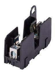
Bussmann modular fuse block, accepts J fuses, 30A, 600V, 1-pole, 14-2 AWG copper or 8-2 AWG aluminum, box lug, 35mm DIN rail or panel mount.
