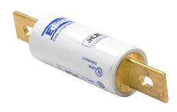
Edison drive fuse, JHL series, Class J, current-limiting, high speed, 80A, 600 VAC, knife blade, feeder/branch, semiconductor protection applications.
