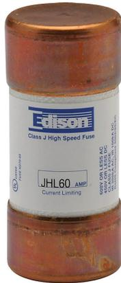
Edison drive fuse, JHL series, Class J, current-limiting, high speed, 60A, 600 VAC, ferrule, feeder/branch, semiconductor protection applications.
