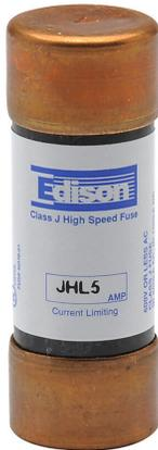
Edison drive fuse, JHL series, Class J, current-limiting, high speed, 5A, 600 VAC, ferrule. Package of 10. Feeder/branch, semiconductor protection applications.
