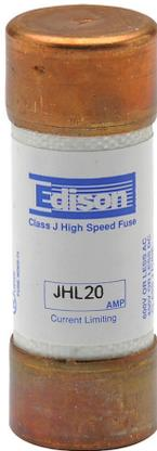
Edison drive fuse, JHL series, Class J, current-limiting, high speed, 20A, 600 VAC, ferrule. Package of 10. Feeder/branch, semiconductor protection applications.
