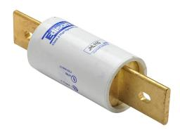
Edison drive fuse, JHL series, Class J, current-limiting, high speed, 110A, 600 VAC, knife blade, feeder/branch, semiconductor protection applications.
