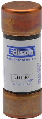
Edison drive fuse, JHL series, Class J, current-limiting, high speed, 10A, 600 VAC, ferrule, feeder/branch, semiconductor protection applications.
