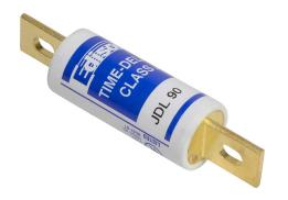
Edison fuse, JDL series, Class J, current-limiting, time-delay, 90A, 600 VAC, knife blade. Package of 5. Feeder/branch protection applications.
