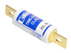
Edison fuse, JDL series, Class J, current-limiting, time-delay, 80A, 600 VAC, knife blade. Package of 5. Feeder/branch protection applications.
