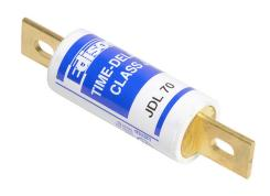
Edison fuse, JDL series, Class J, current-limiting, time-delay, 70A, 600 VAC, knife blade. Package of 5. Feeder/branch protection applications.
