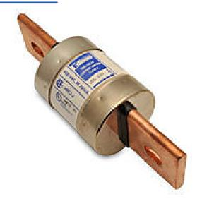
Edison fuse, JDL series, Class J, current-limiting, time-delay, 600A, 600 VAC, knife blade, feeder/branch protection applications.
