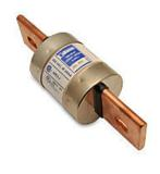
Edison fuse, JDL series, Class J, current-limiting, time-delay, 600A, 600 VAC, knife blade, feeder/branch protection applications.
