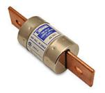
Edison fuse, JDL series, Class J, current-limiting, time-delay, 350A, 600 VAC, knife blade, feeder/branch protection applications.
