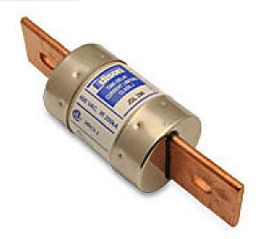
Edison fuse, JDL series, Class J, current-limiting, time-delay, 250A, 600 VAC, knife blade, feeder/branch protection applications.
