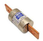
Edison fuse, JDL series, Class J, current-limiting, time-delay, 225A, 600 VAC, knife blade, feeder/branch protection applications.
