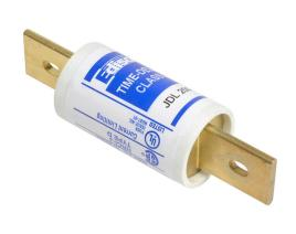
Edison fuse, JDL series, Class J, current-limiting, time-delay, 200A, 600 VAC, knife blade, feeder/branch protection applications.
