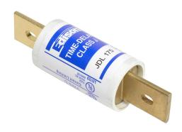
Edison fuse, JDL series, Class J, current-limiting, time-delay, 175A, 600 VAC, knife blade, feeder/branch protection applications.
