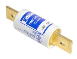
Edison fuse, JDL series, Class J, current-limiting, time-delay, 125A, 600 VAC, knife blade, feeder/branch protection applications.
