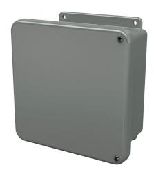
Stahlin J series enclosure, NEMA 1/3R/4X/6P/12, 8 x 8 x 4in (HxWxD), wall mount, fiberglass reinforced polyester, gray, hinged screw cover.
