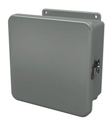
Stahlin J series enclosure, NEMA 1/3R/4X/6P/12, 8 x 8 x 4in (HxWxD), wall mount, fiberglass reinforced polyester, gray, single-door, (1) twist-lock latch.
