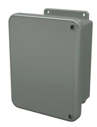
Stahlin J series enclosure, NEMA 1/3R/4X/6P/12, 8 x 6 x 4in (HxWxD), wall mount, fiberglass reinforced polyester, gray, hinged screw cover.
