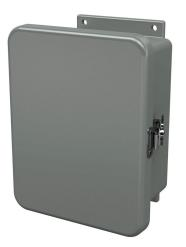
Stahlin J series enclosure, NEMA 1/3R/4X/6P/12, 8 x 6 x 4in (HxWxD), wall mount, fiberglass reinforced polyester, gray, single-door, (1) twist-lock latch.
