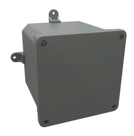
Stahlin NewSentry series enclosure, NEMA 1/2/3/4/4X/12/13, 6 x 6 x 6in (HxWxD), wall mount, PVC, gray, screw cover.
