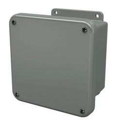
Stahlin J series enclosure, NEMA 1/3R/4X/6P/12, 6 x 6 x 4in (HxWxD), wall mount, fiberglass reinforced polyester, gray, screw cover.
