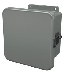
Stahlin J series enclosure, NEMA 1/3R/4X/6P/12, 6 x 6 x 4in (HxWxD), wall mount, fiberglass reinforced polyester, gray, single-door, (1) quick-release latch, padlock hasp and staple.
