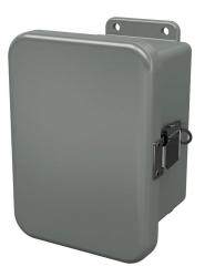
Stahlin J series enclosure, NEMA 1/3R/4X/6P/12, 6 x 4 x 4in (HxWxD), wall mount, fiberglass reinforced polyester, gray, single-door, (1) quick-release latch, padlock hasp and staple.
