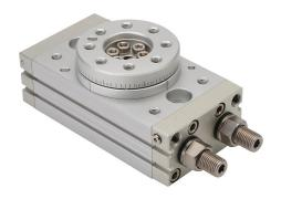
NITRA pneumatic rotary actuator, double acting, size 50, 0 to 190 degrees, rubber bumpers, anodized aluminum body, 1/8in female NPT port(s).
