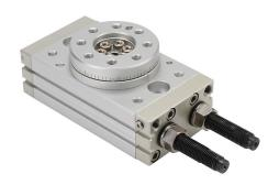
NITRA pneumatic rotary actuator, double acting, size 50, 0 to 190 degrees, shock absorbers, anodized aluminum body, 1/8in female NPT port(s).
