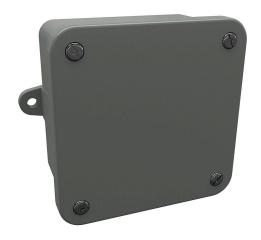
Stahlin NewSentry series enclosure, NEMA 1/2/3/4/4X/12/13, 4 x 4 x 2in (HxWxD), wall mount, PVC, gray, screw cover.
