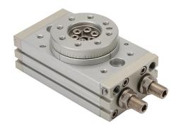
NITRA pneumatic rotary actuator, double acting, size 30, 0 to 190 degrees, rubber bumpers, anodized aluminum body, 1/8in female NPT port(s).
