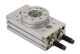
NITRA pneumatic rotary actuator, double acting, size 30, 0 to 190 degrees, shock absorbers, anodized aluminum body, 1/8in female NPT port(s).
