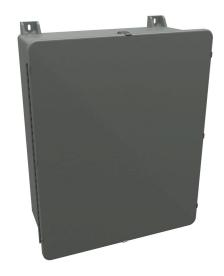
Stahlin J series enclosure, NEMA 1/3/3R/4/4X/12/13, 30 x 24 x 10in (HxWxD), wall mount, fiberglass reinforced polyester, Pantone 428 C glacier gray, single-door, (5) quick-release latches, padlock hasp and staple.
