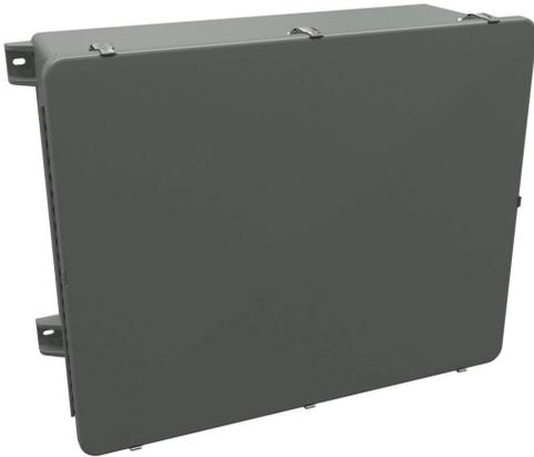
Stahlin J series enclosure, NEMA 1/3/3R/4/4X/12/13, 24 x 30 x 10in (HxWxD), wall mount, fiberglass reinforced polyester, Pantone 428 C glacier gray, single-door, (5) quick-release latches, padlock hasp and staple.
