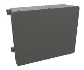
Stahlin J series enclosure, NEMA 1/3/3R/4/4X/12/13, 24 x 30 x 10in (HxWxD), wall mount, fiberglass reinforced polyester, Pantone 428 C glacier gray, single-door, (5) quick-release latches, padlock hasp and staple.
