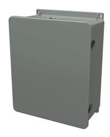
Stahlin J series enclosure, NEMA 1/3/3R/4/4X/12/13, 24 x 20 x 10in (HxWxD), wall mount, fiberglass reinforced polyester, gray, single-door, (4) quick-release latches, padlock hasp and staple.
