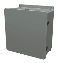
Stahlin J series enclosure, NEMA 1/3/3R/4/4X/12/13, 20 x 20 x 10in (HxWxD), wall mount, fiberglass reinforced polyester, gray, single-door, (4) quick-release latches, padlock hasp and staple.
