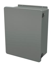
Stahlin J series enclosure, NEMA 1/3R/4X/6P/12, 20 x 16 x 8in (HxWxD), wall mount, fiberglass reinforced polyester, gray, single-door, (2) quick-release latches, padlock hasp and staple.
