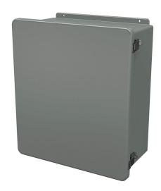
Stahlin J series enclosure, NEMA 1/3R/4X/6P/12, 18 x 16 x 8in (HxWxD), wall mount, fiberglass reinforced polyester, gray, single-door, (2) quick-release latches, padlock hasp and staple.
