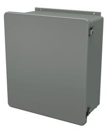
Stahlin J series enclosure, NEMA 1/3R/4X/6P/12, 18 x 16 x 8in (HxWxD), wall mount, fiberglass reinforced polyester, gray, single-door, (2) twist-lock latches.
